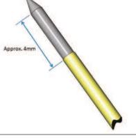
Figure 6: Diagrammatic representation of the 400-micron tapered and stripped tip used for this laser study
